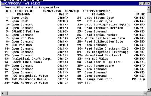
The following screen will appear and step you through entering the current calibration date. Once you enter the year press enter and the program will advance to month and day. Once you have completed entering the calibration date you can verify the calibration date with command "Read Calibration Date"
